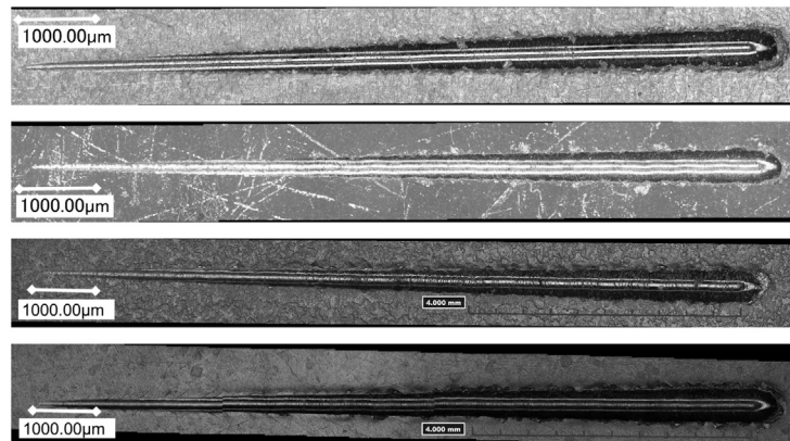
Fig. 9. Residual scratch, from top to bottom: as-plated mid-boron coating; heat-treated mid-boron coating; as-plated high-boron coating; heat-treated high-boron coating.
